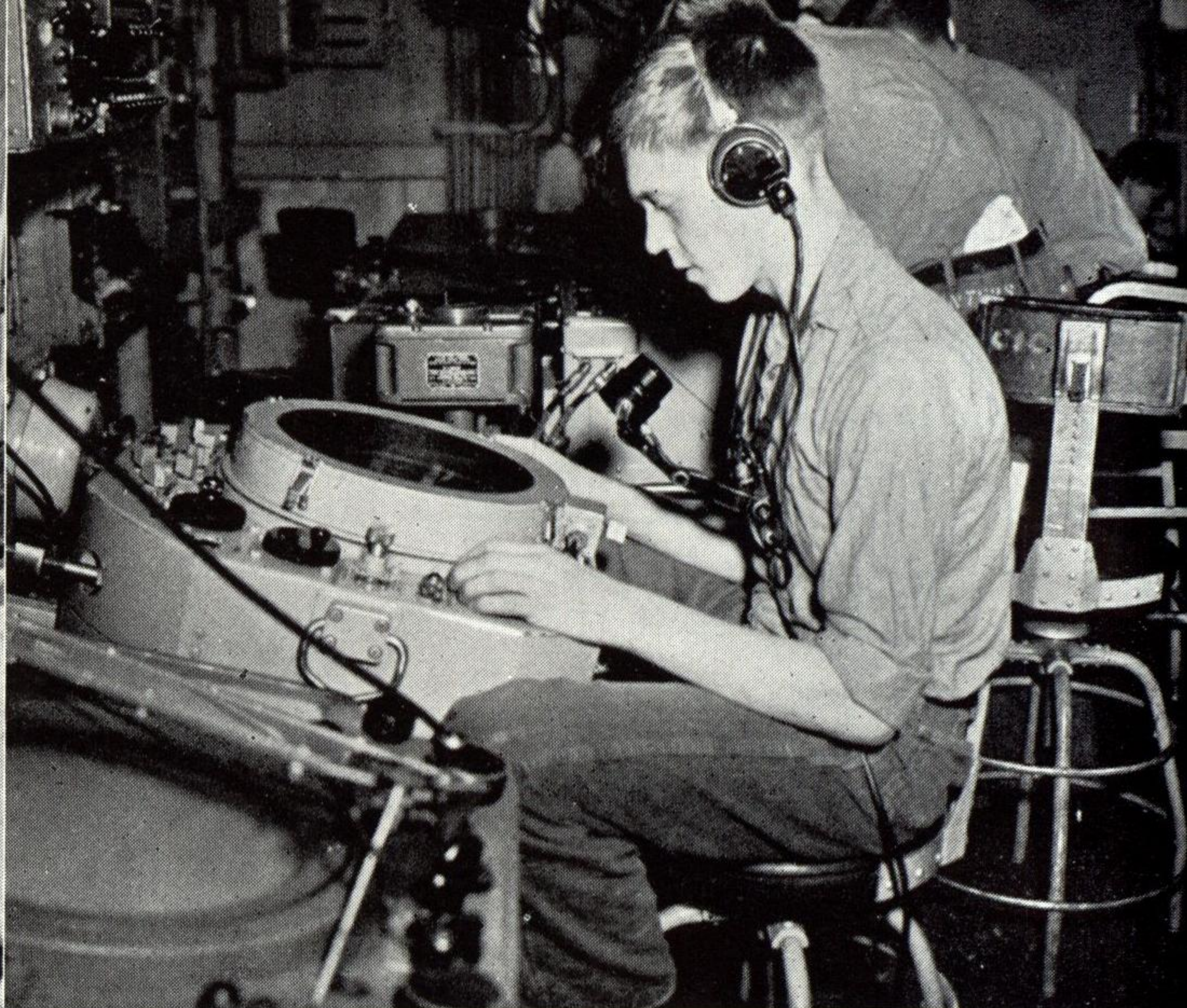
(Above left) CCA directs our aircraft back by radar after the strike. (Above) An air controller scans a radar scope, determining aircraft position course, and speed.
