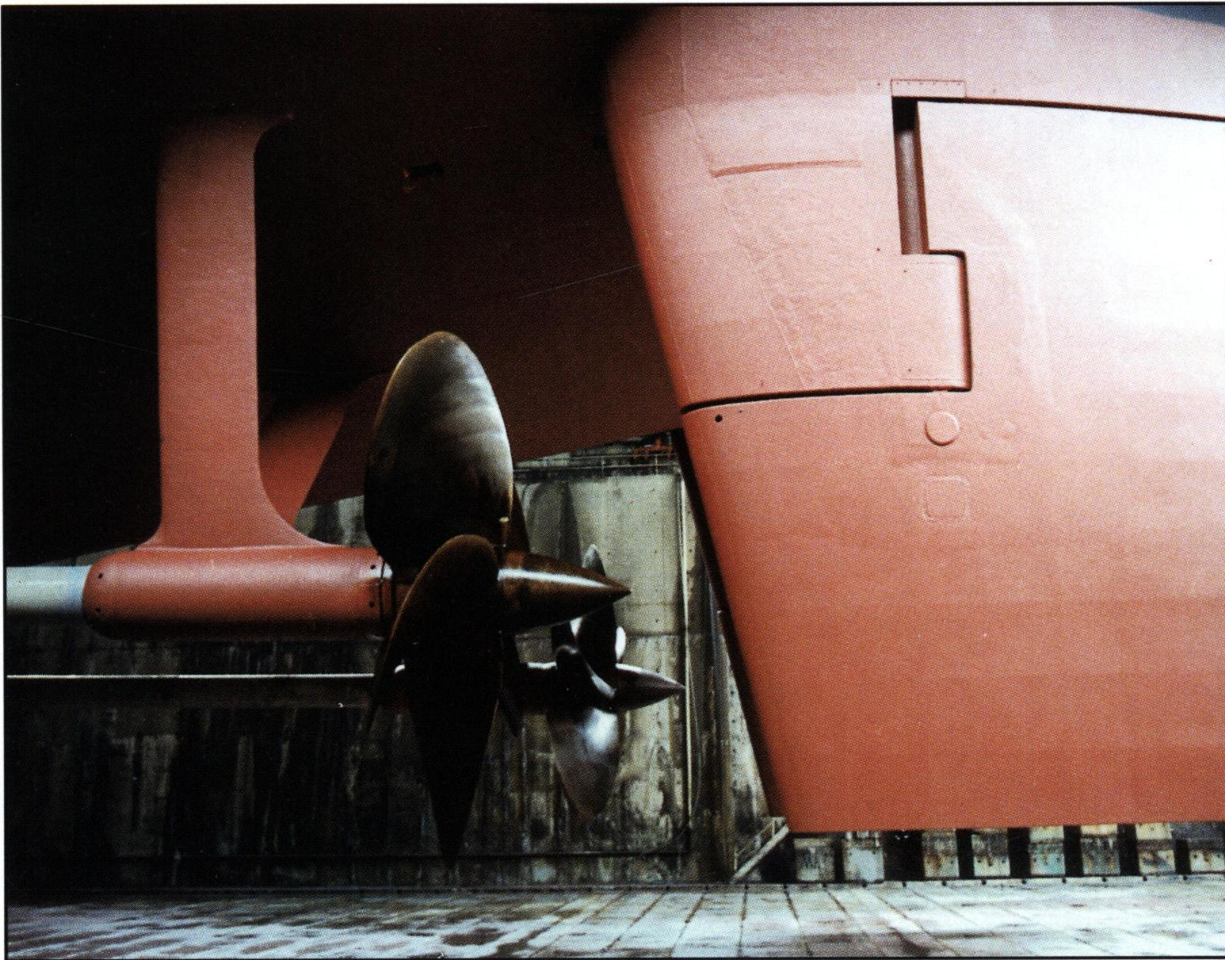
(Above) View of the ship's rudders and two of the 21 feet screws in dry dock.
